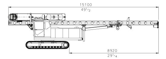
JUNTTAN PM16 with HHK 3A hammer transport dimensions, leader equipped with hinge.
