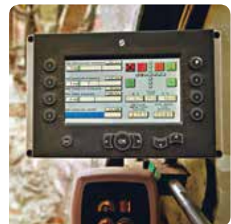
The graphic display of ExcaDrill is user-friendly. The angle and depth measuring system is included. ExcaDrill can be also equipped with a video monitoring camera. This allows the remote visual control of the drilling process on graphic display.
