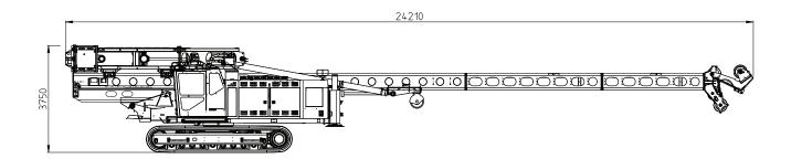
PMx22 transport dimensions with longest available leader configuration (Hydraulic Impact Hammer SHK 100-5).
